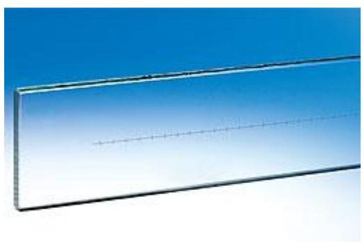
1. Specification: 100mm, 200mm, vernier grid reading: 1mm (national standard : class two).
